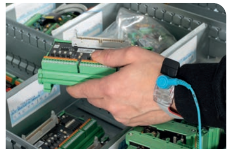
ESD protection system
